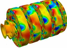
Estimated result of pressure variation on a pump surface (C.Kato, at el, ASME FEDSM2005-77312)
